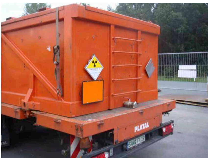
Figure 15: NORM prepared for transportation. Picture courtesy of ExxonMobil.
